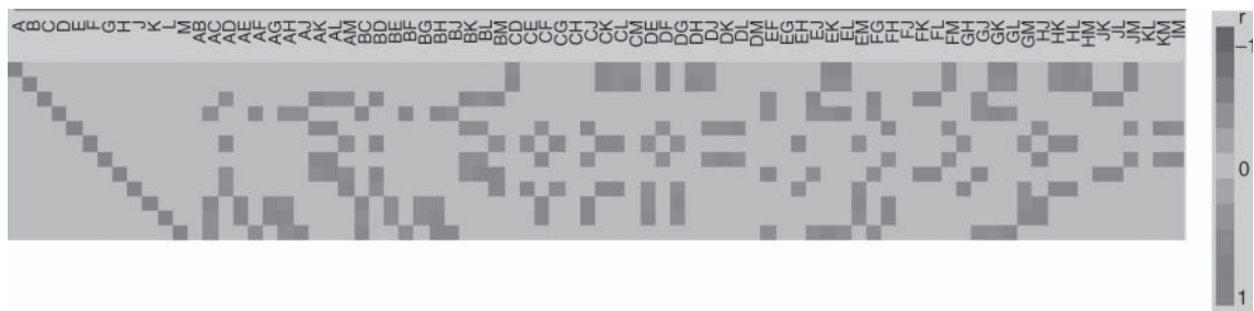
■ FIGURE 9.18 Correlations of main effects and two-factor interactions, no-confounding design for 12 factors in 16 runs
